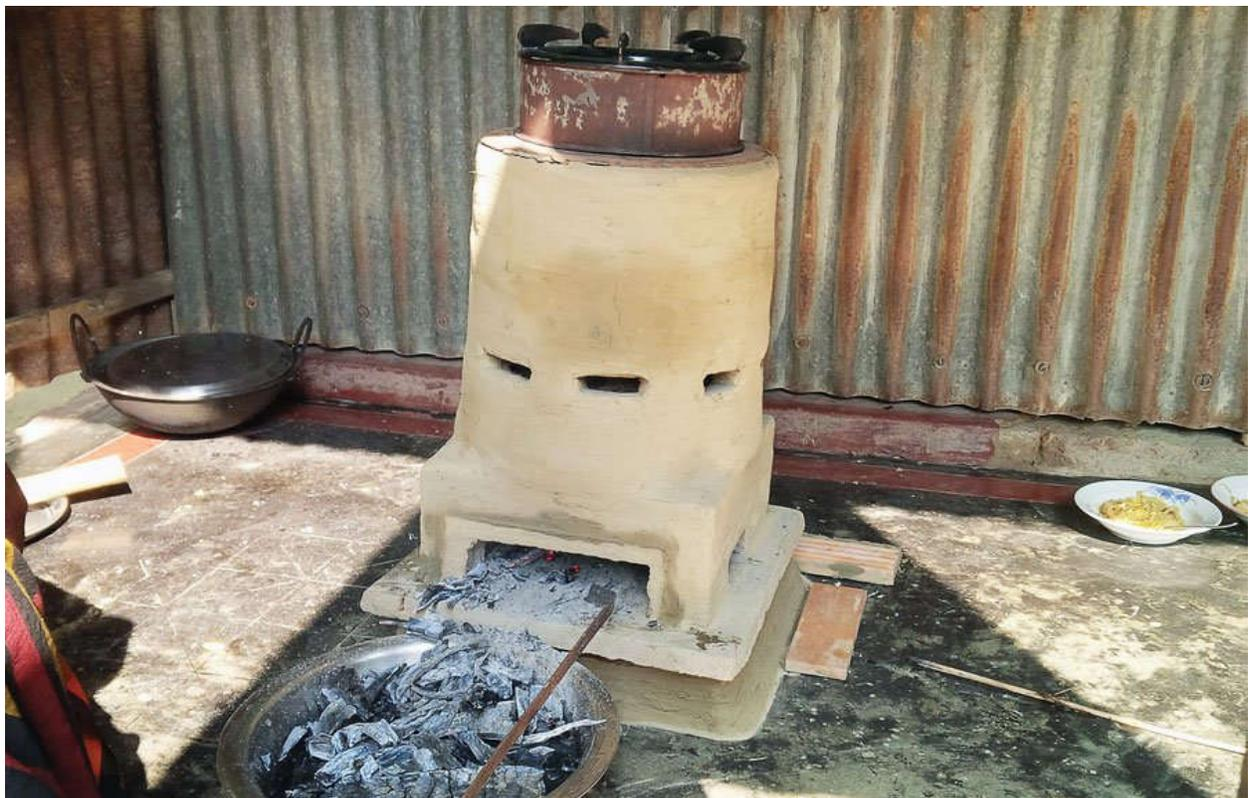
Figure 1 The environment-friendly TLUD stoves, produce a by-product named bio-char which can be the eco-friendly and cheaper alternative to the chemical fertilisers currently used in food production around the country (Abu Siddique)
